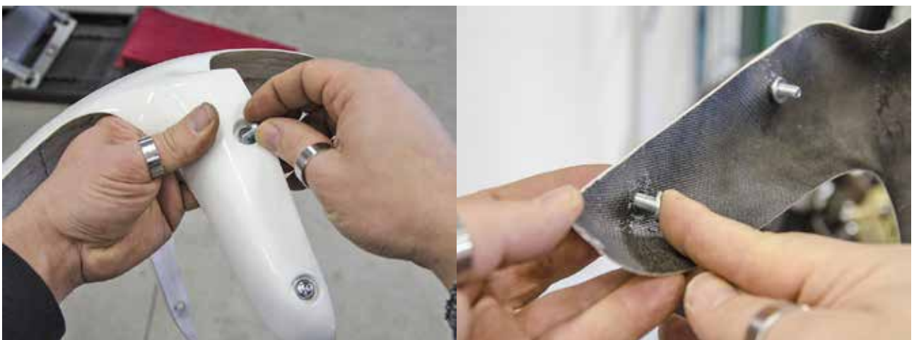
4 Trim new fender, so as to facilitate the passage of the fork outer tube, and drill as photos.
